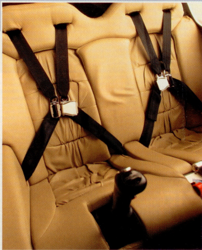
The Eclipse model intended for the civilian market has the PIC position on the left, but the Eclipse aircraft built for the U.S. Air Force Academy puts the pilot on the right. Thus, the throttle is in the student's left hand, as it would be in a jet fighter.
